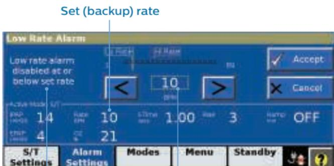
Warning that alarm will not work with current backup rate
