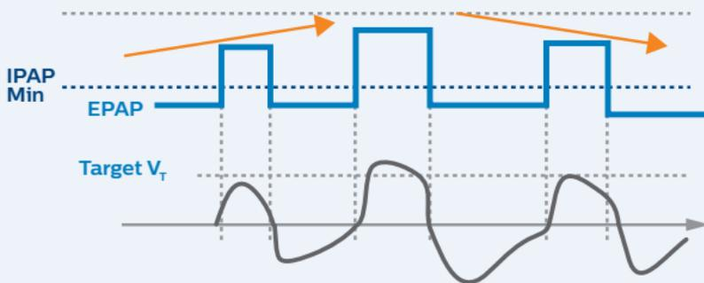
AVAPS automatically adapts pressure support ( $< 2.5 \text{ cmH}_2\text{O}$  per minute) to guarantee an average tidal volume
